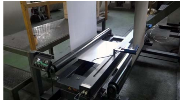
Center Pivot Guider C-1500-BF is used on a Paper Cutting Machine
